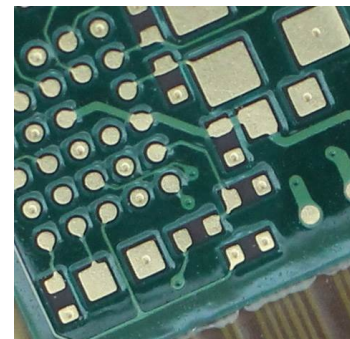
TechniPad ENEPIG - 0.5 mm pitch BGA
