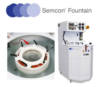
optimum processing for each application by adjusting the sparger, solution flow, and shielding. Each diameter-different cup allows for maximum tool flexibility by being able to run different wafer sizes using a single plating cell, making it extremely versatile and economical. The Semcon Fountain is ideal when setting up an electroplating process for the first time, or when introducing a new metal plating bath to an already existing electroplating process.
