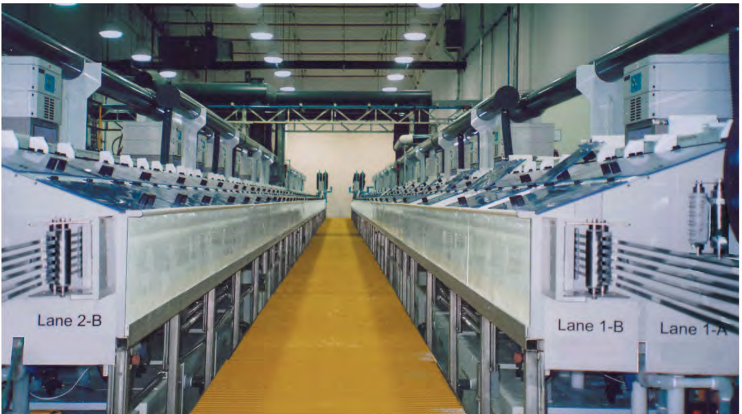
Multi-Strand, Multi-Lane Plating Line
