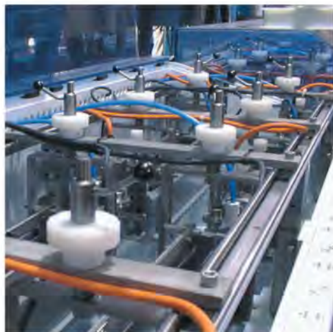
Controlled depth electropolishing station
