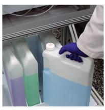
User friendly reagent storage system allows for quick replenishment and level alerts to eliminate downtime.
