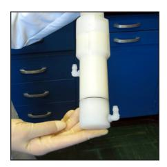
Hardware: The Technic EBA probe has no moving or consumable parts and virtually eliminates the excessive probe maintenance required by competitive instruments. The patented design does not require a classical reference electrode and the automatic sequence creates a clean reproducible working electrode for each measurement. This improves analytical consistency, reduces maintenance, and eliminates down time as well as costs due to worn electrodes.
