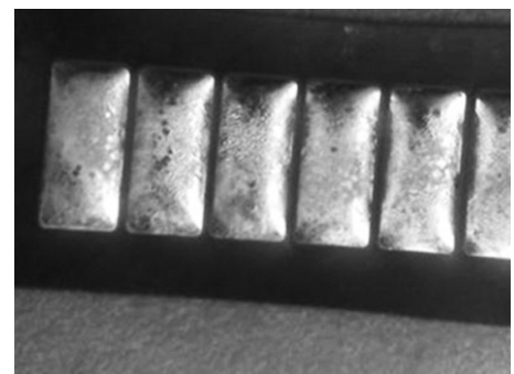
High heat resistance 340°C for 5 sec dipping x 3 times
