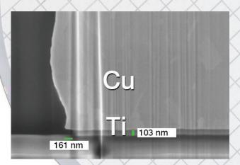
Ti undercut < 0.2µm with overetch of 50%
