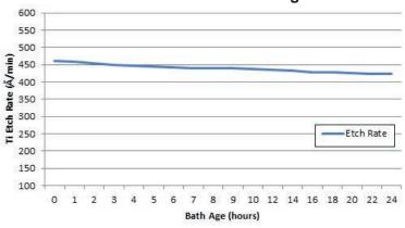
Less than 10% reduction in etch rate at 50°C in a single wafer tool
