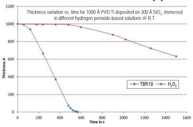
Ti native oxide  $(TiO_2)$  dramatically reduces the Ti etch rate in pure  $H_2O_2$ . The excellent dissolution of  $TiO_2$  in TBR19 enhances and promotes a fast etch rate throughout the process, leading to better etching uniformity and process control.
