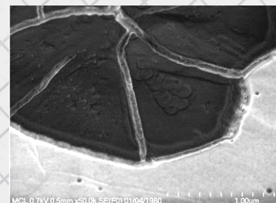
Typical AIF "flower-like" residues prior to TechniClean IK73 cleaning.
