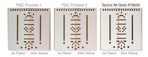
**Cranston RI, USA** – *Techni IM Gold AT8000, Technic's* new non-cyanide gold process released earlier this year, eliminates discoloration of white solder mask when using ENIG as a final finish.
