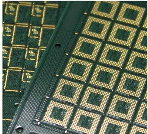
The primary mechanism in Techni IM Gold AT6100 utilizes the Ni as a site for gold reduction but does not remove it from the surface. The additive is not conventional. The reaction stops once the Ni is coated, creating a pore-free surface that allows for a tighter and more controlled deposit.
