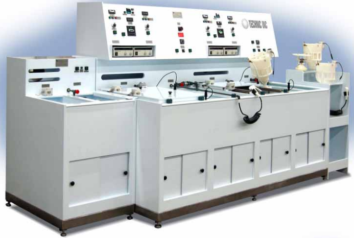
SBE 2-6 with single station activate/rinse and load/unload station
