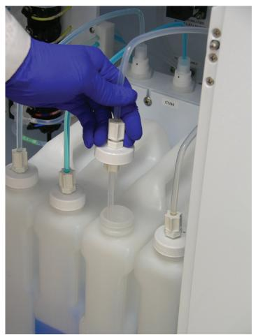
The ACE system houses standard solutions used for automatic calibration adjustments allowing the RTA to run these experiments based a custom schedules tailored for each customer's specific application.
