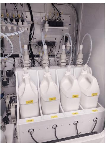
The ACE system houses standard solutions used for automatic calibration adjustments allowing the RTA3D to run these experiments based a custom schedules tailored for each customer's specific application.
