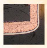
High Speed Nickel Sulfate FFP: High speed process for plating sulfate nickel in an automatic tab plater. The deposit is low stress semi bright and ductile. This process can be used with soluble or insoluble anodes
