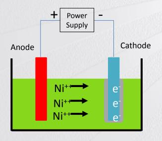
Cathode Current Efficiency = (Exp't wt. gain / theor. wt.)\*100 Anode Current Efficiency = (Anode wt. loss / theor. loss)\*100
