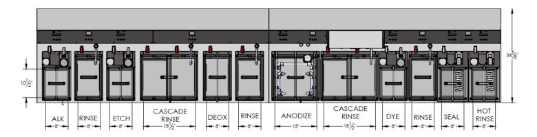
Shown above is the standard configuration for the LAMP. The process sequence represents the MIL-A-8625 Type II and III, Class I & II anodizing.
