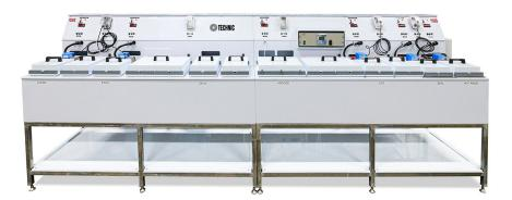
Each unit arrives fully assembled and preconfigured for quick electrical and plumbing connections. Integrated controls, a housed rectifier, and a system-matched chiller ensure precise temperature regulation. Built-in filtration and containment pans provide clean, reliable, and low-maintenance operation in a space-efficient design.
