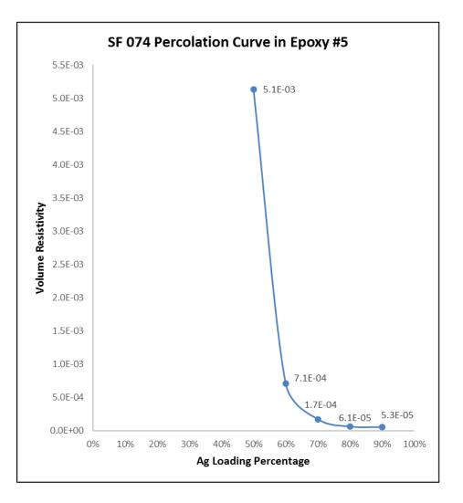
\* Technic's test vehicle, Epoxy #5, consists of Bisphenol F, diaminodiphenyl sulfone cure, reactive diluent, and a coupling agent
