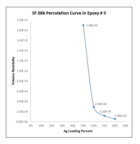
\* Technic's test vehicle, Epoxy #5, consists of Bisphenol F, diaminodiphenyl sulfone cure, reactive diluent, and a coupling agent
