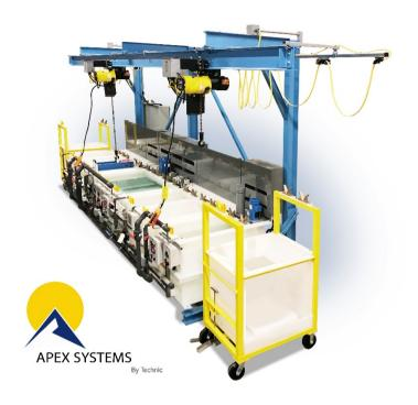
**Module 2:** Anodize and Post-treatment – 6 tanks (5 polypro, 1 SS) 24" x 24" x 24" deep, two heaters, agitation, water, drain.
