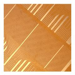
TechniMask UV-SR2 is a liquid, UV-curable solder mask material, specifically designed for flexible, flex-rigid and rigid circuits. It is halogen free and meets RoHS and UL94 V-0 flammability specifications. Its excellent cosmetic appearance, encapsulation, and resolution without skips and bleed, as well as good flexibility and adhesion to various substrates, makes it a cost effective alternative to photodefinable coverlays or solder masks.
