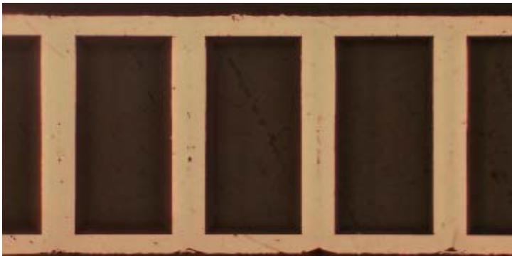
260 \mu\text{m} x 40 \mu\text{m} through-hole via fill on glass substrate
